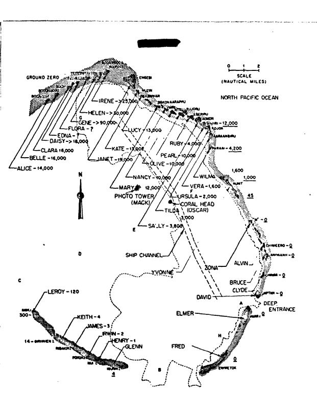
Fig. 10.1 — Mike shot, H + 24 hr. Underlined readings are ground values in milliroentgens per hour; other readings are helicopter readings 25 ft above ground in milliroentgens per hour.
