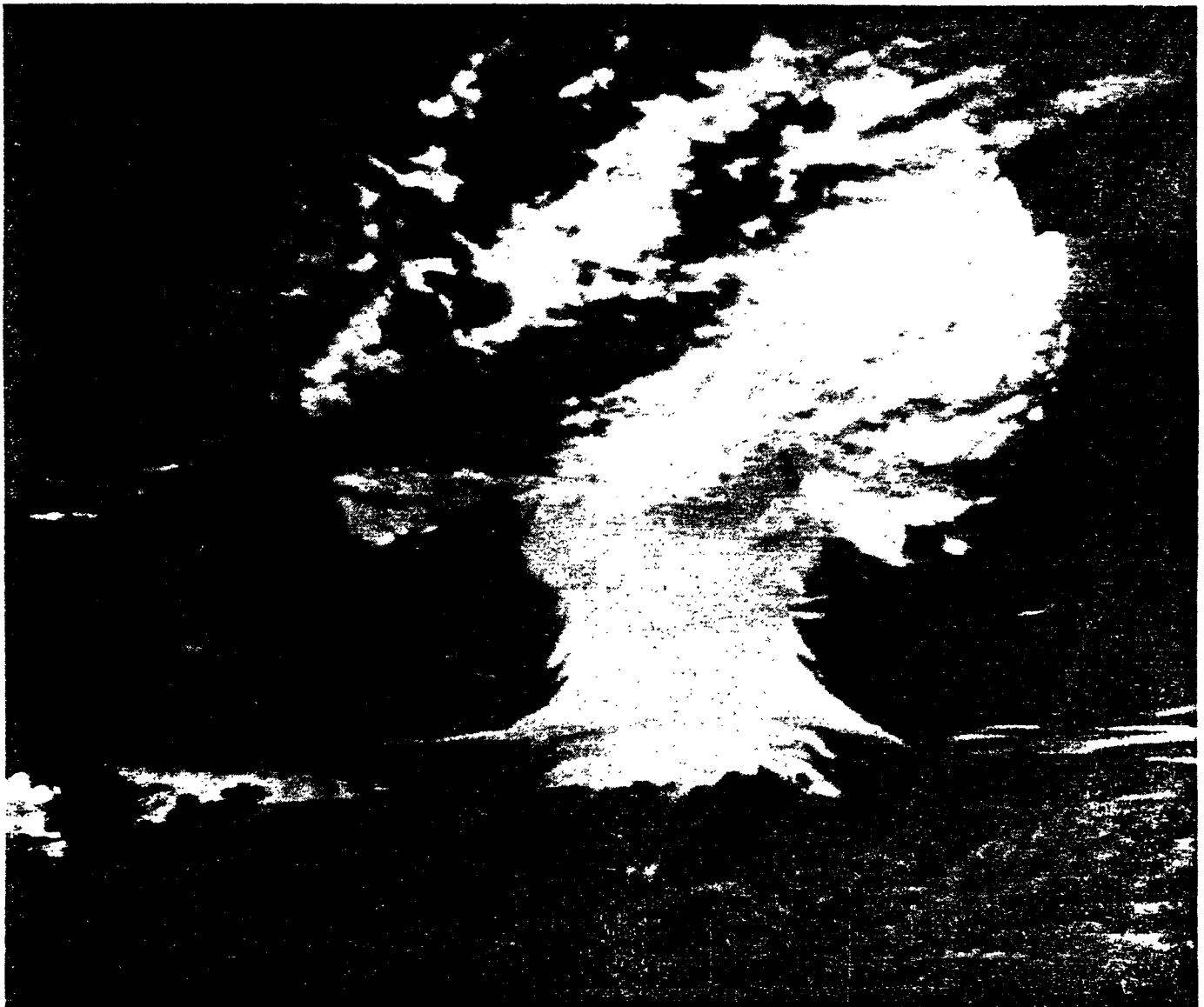
FIRST SUPERBOMB TEST in which a large thermonuclear, or fusion, explosion was successfully ignited by a comparatively small fission explosion took place at the Eniwetok Proving Ground in the Marshall Islands on November 1, 1952 (local time). The device, with the code name Mike, released an amount of energy equivalent
